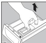
Detergent can also accumulate inside the drawer recess: clean it with an old toothbrush. Refit the drawer after cleaning.
